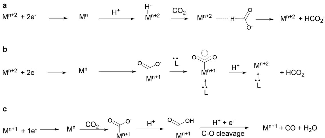
Scheme 3 (a and b) Pathways for the two-electron  $\text{CO}_2$  reduction to formate involving a metal-hydride (a) or a metal carboxylate (b) as an intermediate. Pathway (b) has been shown to be followed with **Fe1** in the presence of tertiary amines in DMF solutions.<sup>40</sup> (c) Pathway for the two-electron  $\text{CO}_2$  reduction to CO.  $\text{M}^n$  is the active form of the catalyst.
