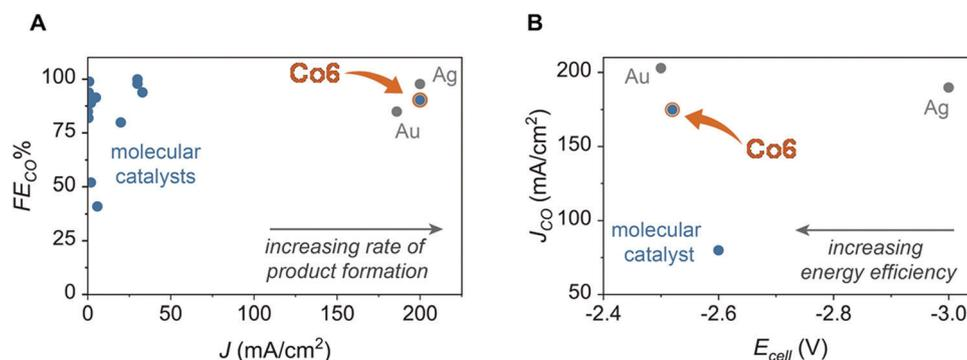
Fig. 12 Comparison of selectivity (A) and activity (B, partial current density) for CO production with **Co6** inserted in a zero-gap membrane flow reactor and previous molecular and heterogeneous CO<sub>2</sub> reduction electrocatalysts (adapted from ref. 118 with permission from AAAS, copyright 2019).
