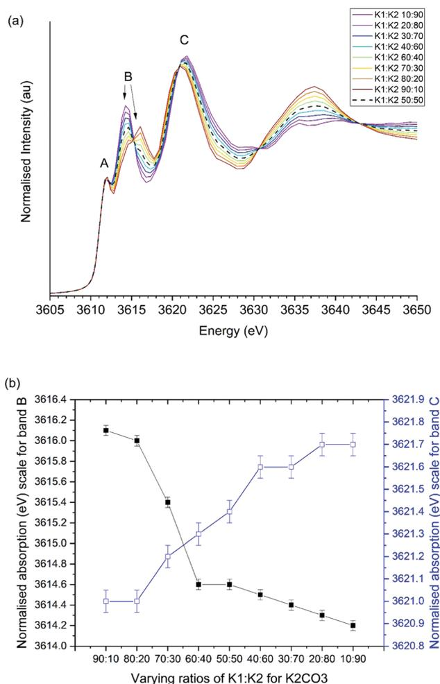
Fig. 9 Influence of K1:K2 ratio on simulated XANES spectra of K<sub>2</sub>CO<sub>3</sub>. (a) Simulated XANES, (b) position of observed bands B and C.
