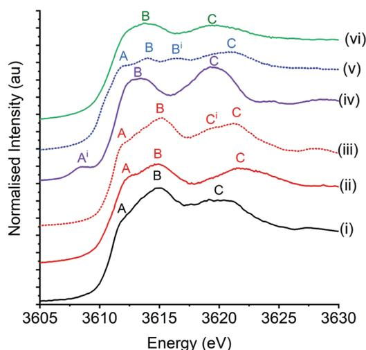
Fig. 2 Potassium K-edge XANES of  $K/\alpha-Al_2O_3$  and standards. (i)  $K/\alpha-Al_2O_3$  (ii)  $K_2CO_3$ , (iii)  $KHCO_3$ , (iv)  $K_2O$ , (v)  $K(CH_3CO_2)$  and (vi)  $KOH \cdot xH_2O$ . Features;  $A^1$  is  $1s \rightarrow 3d$ ,  $A$  is  $1s \rightarrow 4s$ ,  $B$  and  $B^1$  is  $1s \rightarrow 4d$  and  $C/C^1$  is multiple scattering resonances.
