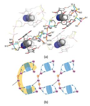
Fig. 3 The exo-coordinated mercury( ${\mbox{\tiny II}}$ ) bromide complex [Hg<sub>6</sub>Br<sub>12</sub> (CH<sub>3</sub>CN@L)<sub>2</sub>]<sub>n</sub> (**2**): (a) the 1-D polymeric structure (the asymmetric unit is shown with the labelling) and (b) the connectivity pattern showing the linkage of the C-shaped dimers (terminal Br atoms are omitted). Symmetry operation A: -1 + x, -y, -0.5 + z.
