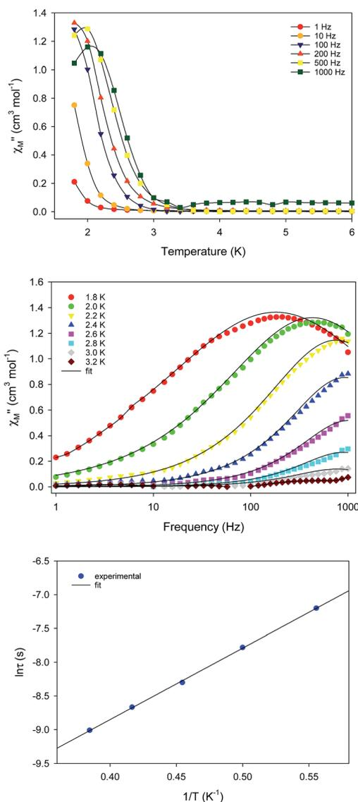
Fig. 4 (top) Out-of-phase ( $\chi_{\text{M}}''$ ) ac magnetic susceptibility signals for **1-w** at zero dc field; the solid lines are guides for the eye. (middle) Frequency dependence of  $\chi_{\text{M}}''$  at different temperatures for **1-w** at zero dc field; the solid lines are best fits to the generalized Debye model. (bottom) Arrhenius plot of  $\tau$  versus  $1/T$  for **1-w**; the solid line is the best fit as described in the text.
