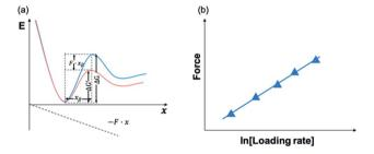
Fig. 4 Schematic figures of energy landscape (a) and force-loading rate dependency (b). Applied force can tilt the energy landscape and lower the energy barrier. By fitting force-loading rate relationship, dissociation rate and distance to transition state can be extracted
