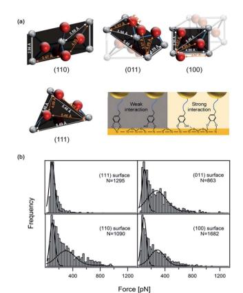
Fig. 6 Influence of surface atom arrangement on DOPA adhesion. Schematics of different rutile surface atom arrangements and proposed binding modes of DOPA-surface interactions (a). Rupture force histograms observed from DOPA and different rutile surfaces (b). Copyright (2017) Wiley. Used with permission from ref. 16.
