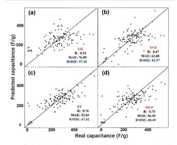
Fig. 3 Statistical performance of each ML model by comparing the predicted capacitance from ML models (y-axis) and the real experimental capacitance (x-axis). (a) LR, (b) SVR, (c) RT, and (d) MLP. If the dot for a certain carbon electrode lies on the solid line, it means that the predicted capacitance and input (experimental) capacitance are the same.
