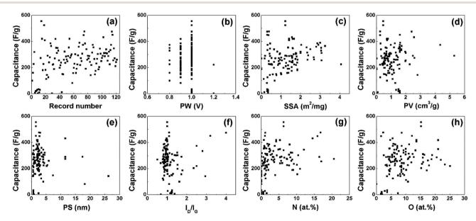
Fig. 2 Input data with different variables, 121 sets of capacitances for different carbon-based electrodes (a). The relationship between the capacitance and potential window (b), specific surface area (c), pore volume (d), pore size (e), ratio of I<sub>D</sub>/I<sub>G</sub> (f), N-doping percentage (g), and Odoping percentage (h).
