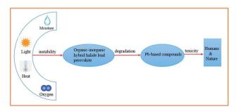
Fig. 1 Schematic of the instability and toxicity of organic-inorganic hybrid halide lead perovskite compounds.
