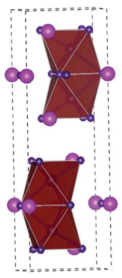
Fig. 9 Crystal structure of  $A_3B_2I_9$  perovskites. The magenta spheres represent the Cs atoms, blue spheres represent the trivalent metal atom (Bi, Sb atom), and purple spheres represent the I atom.
