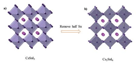
Fig. 8 (a) Crystal structure of CsSnI<sub>3</sub>. (b) Crystal structure of Cs<sub>2</sub>SnI<sub>6</sub>. Consulting from ref. 79.
