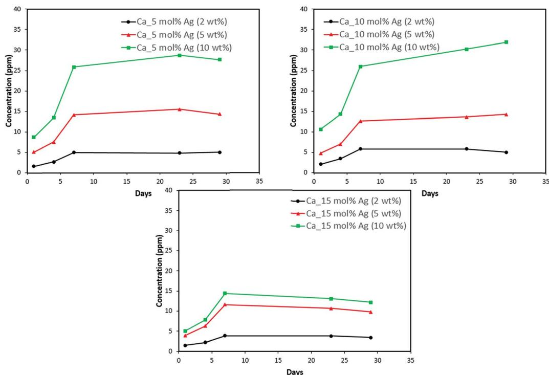
Fig. 10 Calcium release from adhesive resin disc specimens containing 5, 10 and 15 mol% silver with different weight fractions of silver-ACP.
