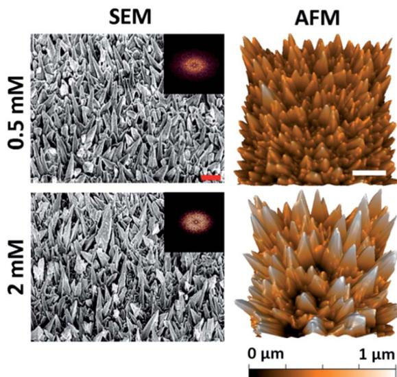
Fig. 3 Native surface data for the  $\text{Pb}^+$  concentration series: column (1) SEM ( $45^\circ$  tilted) and column (2) AFM images of the gold nanospike surfaces for 0.5 and 2 mM  $\text{Pb}(\text{CH}_3\text{COO})_2$ . The 2D-FFT data is shown for the top-down SEM images (see Fig. S5†). The red and white scale bars are 200 nm and 1  $\mu\text{m}$ , respectively.
