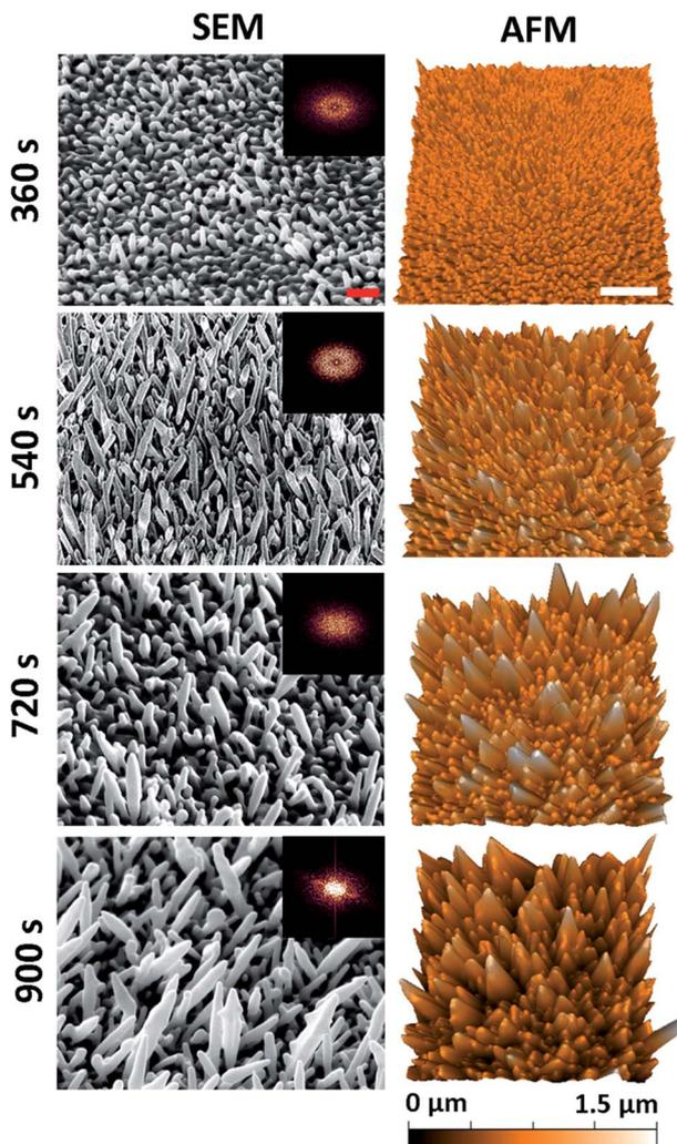
Fig. 1 Native surface data for the nanopike deposition series: column (1) SEM (45° tilted) and column (2) AFM images of the gold nanopike surfaces as a function of electrodeposition time. The red and white scale bars are 200 nm and 1 μm, respectively. 2D-FFT data (insets) are shown for the top-down SEM images (see Fig. S2†).
