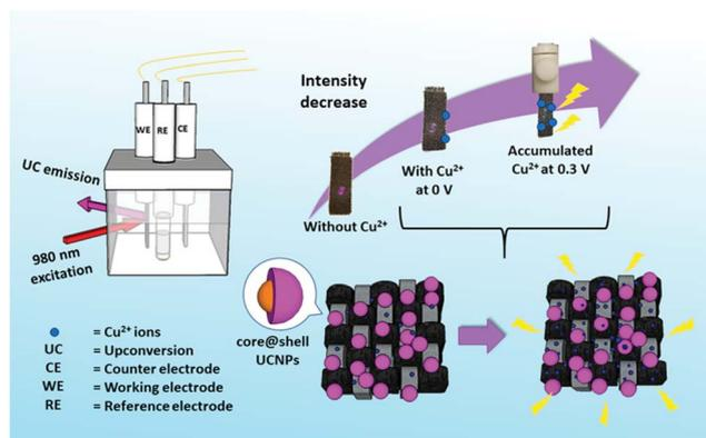
Fig. 1 A schematic diagram showing the CFC-UCNP probe for  $\text{Cu}^{2+}$  ion sensing under the E-chem assistance.
