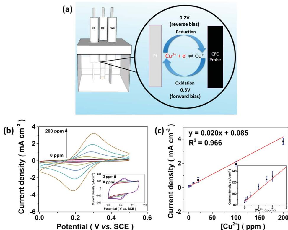
Fig. 4 (a) A diagram illustrating the E-chem processes on the CFC-UCNP probe. (b) CV curves of the CFC-UCNP probe in response to 0–200 ppm  $\text{Cu}^{2+}$  ions recorded within the potential window of 0–0.5 V at  $100 \text{ mV s}^{-1}$ . (c) The linear relationship between the E-chem signals and  $[\text{Cu}^{2+}]$  obtained at 0.3 V. The insets are the enlarged plots for 0–2 ppm  $\text{Cu}^{2+}$  ions.
