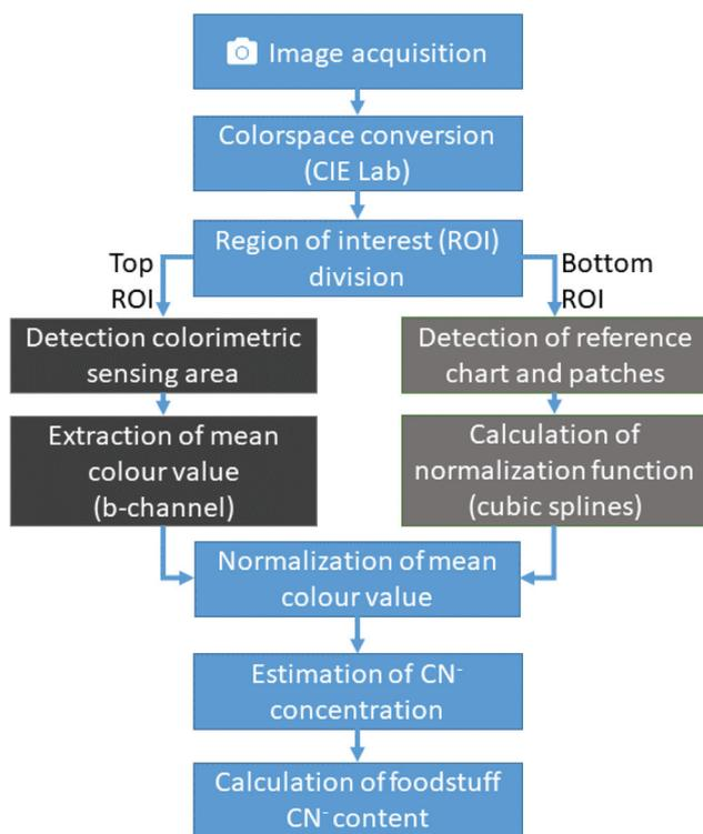
**Fig. 4** Algorithm for image acquisition and processing. The top and bottom regions of interest (ROI) are processed independently and then results combined to normalize sensing area colour and estimate cyanide ( $\text{CN}^-$ ) concentration in the sample and foodstuff.
