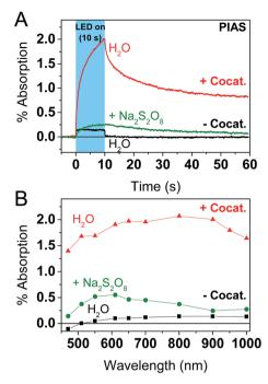
Fig. 4 PIAS results for GaN:ZnO in  $H_2O$  (black traces), GaN:ZnO in aqueous  $Na_2S_2O_8$  (green traces), and GaN:ZnO/Rh<sub>2-y</sub>Cr<sub>y</sub>O<sub>3</sub> in  $H_2O$  (red traces). (A) Kinetics monitored at 900 nm. The blue shaded area correspond to the temporal pulse width of the 365 nm LED excitation (10 mW cm<sup>-2</sup>). (B) PIAS spectra obtained following 10 seconds of irradiation.  $[Na_2S_2O_8] = 10$  mM.
