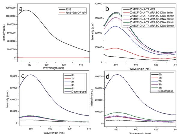
Fig. 2 (a) Fluorescence of RhB was quenched upon addition of ZrMOF nanoparticles. (b) Fluorescence of TAMRA was quenched upon conjugation with ZrMOF nanoparticles but recovered after adding complementary DNA. (c) Quenching stability of ZrMOF-Library-TAMRA in cell culture medium DMEM. (d) Quenching stability of ZrMOF-aptamer-TAMRA in cell culture medium DMEM.
