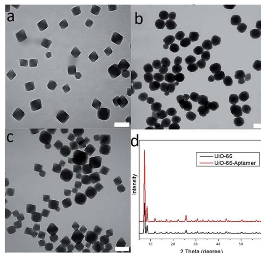
Fig. 5 (a) TEM of UiO-66 nanoparticles before aptamer conjugation in DMF. (b) TEM of HfMOF nanoparticles after phosphate-terminal aptamer conjugation in water. (c) TEM of UiO-66 nanoparticles after phosphate-terminal aptamer conjugation in water. (d) Powder X-ray diffraction of UiO-66 nanoparticles before (black) and after phosphate-terminal aptamer conjugation (red). Scale bar: 200 nm.
