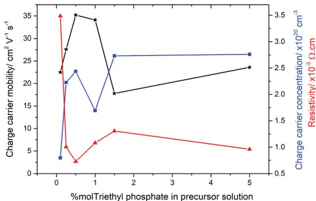
Fig. 5 Electrical properties for the P-doped SnO<sub>2</sub> films as obtained by Hall effect measurements.
