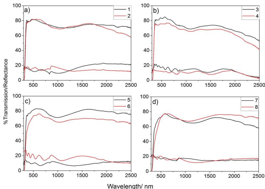
Fig. 4 UV/vis/NIR spectra for P-doped SnO<sub>2</sub> films; (a) undoped SnO<sub>2</sub> (1) and 0.1 mol% P:SnO<sub>2</sub> (2); (b) 0.25 mol% P:SnO<sub>2</sub> (3) and 0.5 mol% P:SnO<sub>2</sub> (4); (c) 1 mol% P:SnO<sub>2</sub> (5) and 1.5 mol% P:SnO<sub>2</sub> (6); and (d) 5 mol% P:SnO<sub>2</sub> (7) and 7.5 mol% P:SnO<sub>2</sub> (8). In all cases the films showed high transmission (ca. 80%) and low reflection (<20%). All films deposited by AACVD at 550 °C using air as carrier gas.
