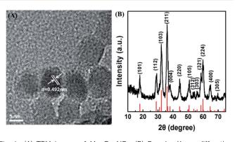
Fig. 1 (A) TEM image of Mn<sub>3</sub>O<sub>4</sub> NPs. (B) Powder X-ray diffraction pattern of Mn<sub>3</sub>O<sub>4</sub> NPs (the red lines at the bottom mark the reference pattern of hausmannite Mn<sub>3</sub>O<sub>4</sub> from the JCPDS database, card no. 24-0734).
