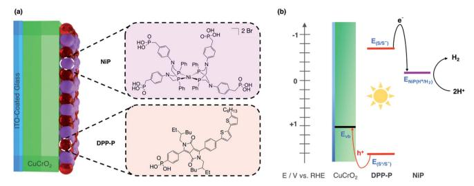
Fig. 1 (a) Dye (DPP-P) and catalyst (NiP) co-immobilised on the CuCrO<sub>2</sub> electrode with their molecular structures. (b) Energy diagram showing movement of electrons with black and holes with red arrows. S represents the dye sensitiser where  $E_{(S/S^-)}$  is the ground state reduction potential and  $E_{(S^*/S^-)}$  is the reduction potential in the excited state.  $E_{NiP(H^+/H_2)}$  is the catalytic onset potential for NiP and  $E_{vb}$  is the CuCrO<sub>2</sub> valence band
