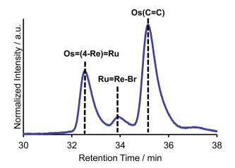
Fig. 2 Size-exclusion chromatogram measured after the reaction for the synthesis of Os=(4-Re)=Ru.
