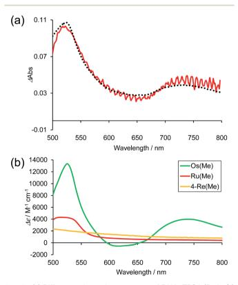
Fig. 10 (a) Difference absorption spectrum of DMA–TEOA (5:1 v/v) solution containing Os–(4-Re)–Ru (0.01 mM) and BIH (0.1 M) after irradiation at  $\lambda_{\rm ex}=480$  nm for 1 min under Ar atmosphere (red line), and the fitting spectrum with 15% Os(Me) and 85% 4-Re(Me) (black line). (b) The difference absorption spectra between the OERS and the non-reduced complexes of Os(Me) (green),  $^{10}$  Ru(Me) (red)  $^{40}$  and 4-Re(Me) (orange).  $^{40}$
