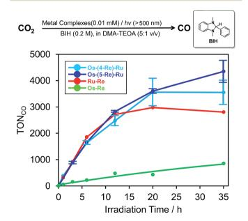
Fig. 7 Time courses of the TON of CO formation during photocatalytic reactions ( $\lambda_{ex} > 500$  nm) using a mixture of DMA and TEOA (5 : 1 v/v) containing 0.2 M BIH and metal complexes (sky blue: Os-(4-Re)-Ru, blue: Os-(5-Re)-Ru, red: Ru-Re, yellow-green: Os-Re). The concentration of each complex was 0.01 mM.
