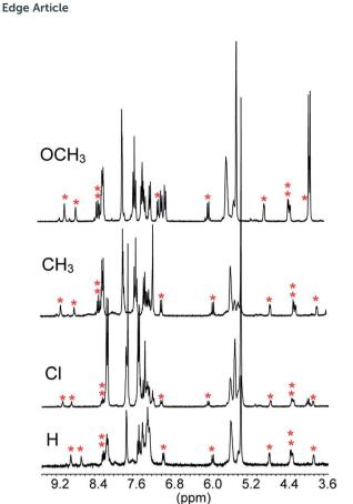
Fig. 1 Portions of the  $^1$ H NMR spectra (CD<sub>2</sub>Cl<sub>2</sub>, 25 °C) recorded in the course of the reaction of 5 mM 1 with equimolar amounts of acid 2 (X = H, Cl, CH<sub>3</sub> and OCH<sub>3</sub>) after 3.5, 2.5, 7.5 and 44.5 min from the start, respectively. The signals marked with an asterisk are proposed to belong to ten of the twelve protons of the two non-equivalent phenanthroline units in B''. The peak at 5.30 ppm is due to CHDCl<sub>2</sub>.
