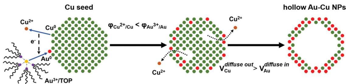
**Scheme 1** Growth mechanism of hollow Au–Cu NPs.
