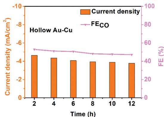
**Fig. 4** Chrono-amperometry results of hollow Au–Cu NP/C tested for CO<sub>2</sub>RR at -0.7 V (vs. RHE) for 12 h.
