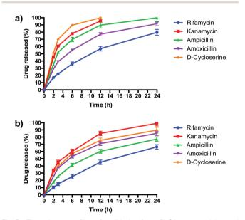
Fig. 5 The release profiles of antibiotics from PLGA nanoparticles and PLGA/DOTAP nanoparticles. In vitro release profiles of different antibiotics from (a) PLGA nanoparticles and (b) PLGA/DOTAP nanoparticles in PBS (pH 7.4) for 24 h at 37 °C (n = 5, mean  $\pm$  S.D).
