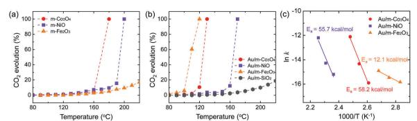
Fig. 3 Catalytic activity of full-oxidation of methanol to  $CO_2$  as a function of temperature for (a) pure mesoporous oxides and (b) Au nanoparticles supported on mesoporous oxides. (c) Arrhenius plots of the rate of CO production on the Au/m-oxide catalysts.
