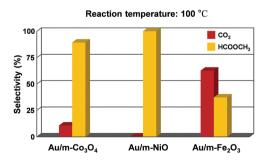
Fig. 4 Selectivity showing the fraction of methanol converted to carbon dioxide and methyl formate at 100  $^{\circ}$ C for Au-supported mesoporous oxides (Co<sub>3</sub>O<sub>4</sub>, NiO, and Fe<sub>2</sub>O<sub>3</sub>).
