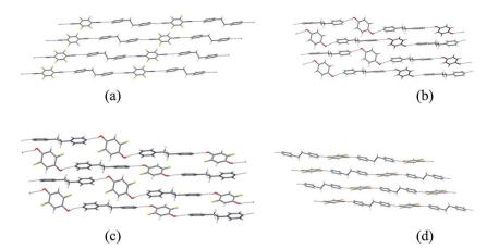
Fig. 1 Crystal structures of co-crystals: (a) XB network  $1 \cdot 3$ , (b) HB network  $2a \cdot 3$ , (c) HB network  $2b \cdot 3$ , (d) HB network  $2c \cdot 3$ . The molecule of 2b (in (c)) exhibits 50 : 50 F/H disorder at the 2- and 5-positions; disordered H atom sites are not shown. The crystal structures of  $1 \cdot 3$  and  $2a \cdot 3$  have been previously reported<sup>37</sup> and are consistent with the structures determined herein.
