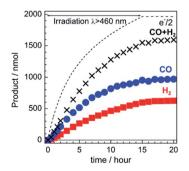
Fig. 4 Time courses of the chemical products (CO and H<sub>2</sub>) and a half amount of electrons passing through the RuRe/CuGaO<sub>2</sub> photocathode under continuous visible-light irradiation ( $\lambda_{\rm ex}$  > 460 nm) at -0.3 V vs. Ag/AgCl. A 50 mM aqueous solution of NaHCO<sub>3</sub> (pH 6.6) that was saturated with CO<sub>2</sub> was used as the electrolyte.
