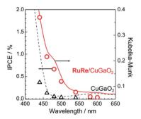
Fig. 2 Dependence on wavelength of the incident-photon-to-current efficiencies of the RuRe/CuGaO2 (red circles) and bare CuGaO2 (black triangles) electrodes at -0.3 V vs. Ag/AgCl. An aqueous solution containing 50 mM NaHCO3 saturated with CO2 was used as the electrolyte (pH 6.6). The diffuse reflectance spectra of these electrodes are also shown: RuRe/CuGaO2 (red solid line) and CuGaO2 (black broken line).
