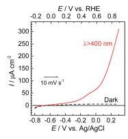
Fig. 7 Current–potential curves of the  $CoO_x/TaON$  photoanode under continuous visible-light irradiation ( $\lambda_{ex} > 400$  nm) and under dark conditions. A 50 mM aqueous solution of NaHCO<sub>3</sub> (pH 6.6) saturated with CO<sub>2</sub> was used as the electrolyte.
