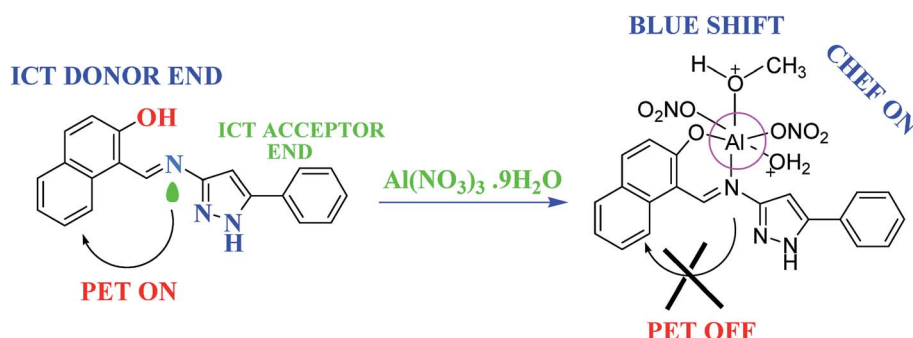
Fig. 8 Probable mechanistic pathway for sensing Al(III) ions. 108
