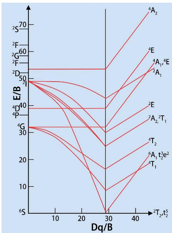
Fig. 2 Tanabe–Sugano diagram for the  $d^5$  electron configuration.<sup>19</sup>
