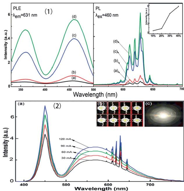
Fig. 7 (1) Excitation and emission spectra of the  $\text{Na}_2\text{SiF}_6:\text{Mn}^{4+}$  phosphor with HF concentrations of (a) 10, (b) 20, (c) 30, and (d) 40 wt%. (2) Luminescence spectra based on the  $\text{Na}_2\text{SiF}_6:\text{Mn}^{4+}$  phosphor under various drive currents.<sup>36</sup>
