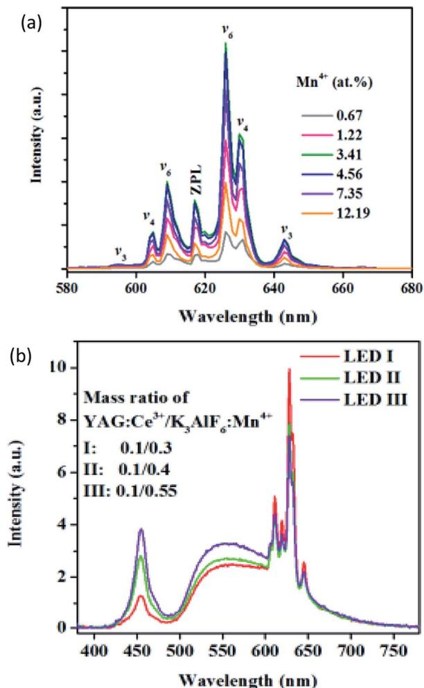
Fig. 8 (a) Concentration dependent emission spectra of  $\text{K}_3\text{AlF}_6:\text{Mn}^{4+}$ . (b) Electroluminescence spectra of prototype LEDs, employing  $\text{K}_3\text{AlF}_6:\text{Mn}^{4+}$  as the red converter component, commercial yellow  $\text{YAG}:\text{Ce}^{3+}$  and a blue InGaN chip at a 40 mA drive current.<sup>42</sup>
