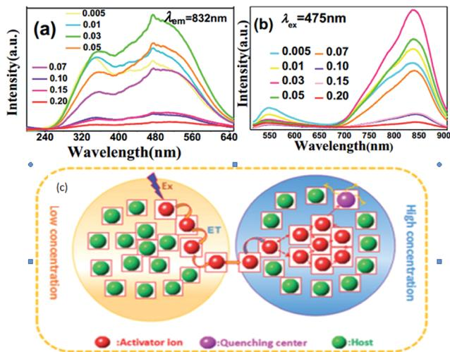
Fig. 11 (a) PLE and (b) PL spectra of the LZG: $x\text{Mn}^{2+}$  samples ( $0 < x < 0.2$ ). (c) A diagram of the concentration quenching process.<sup>52</sup>
