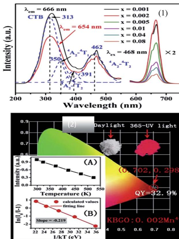
Fig. 6 (1) PL spectra of  $\text{K}_2\text{BaGe}_8\text{O}_{18}:\text{Mn}^{4+}$  with different concentrations, and PL excitation spectra of the  $\text{K}_2\text{BaGe}_8\text{O}_{18}:0.002\text{Mn}^{4+}$  sample monitored at 666 nm and 654 nm. (2) Chromatic CIE coordinates, quantum yields and variation of emission intensity depending on the temperature of the representative  $\text{K}_2\text{BaGe}_8\text{O}_{18}:\text{Mn}^{4+}$ .<sup>32</sup>
