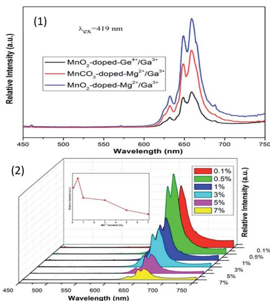
Fig. 5 (1) PL properties of samples with different Mn sources and doped sites. (2) PL under 419 nm excitation of the  $\text{Mg}_3\text{Ga}_2\text{GeO}_8:x\% \text{Mn}^{4+}$  series phosphors.<sup>31</sup>
