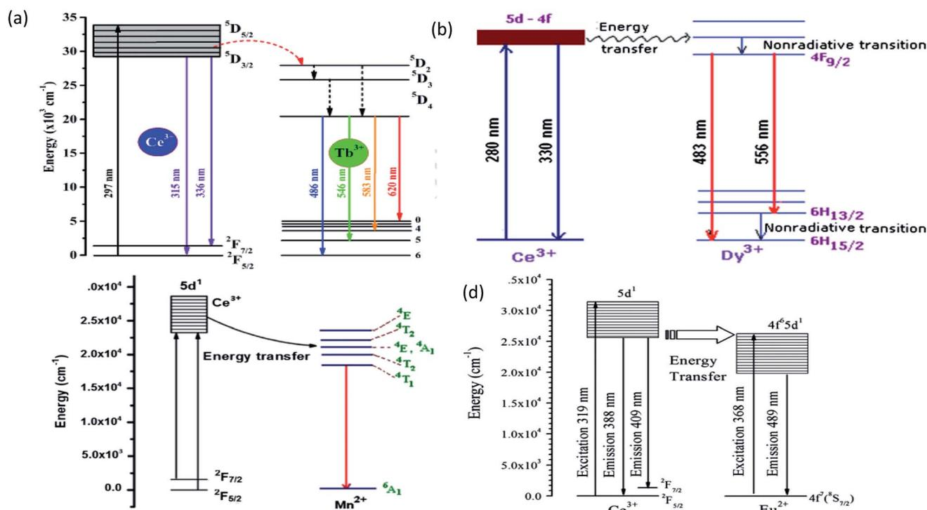
Fig. 14 (a) The schematic energy level diagram for the energy transfer process in the  $\text{BaMgF}_4:\text{Ce}^{3+}, \text{Tb}^{3+}$  phosphors.<sup>75</sup> (b) Energy level diagram of  $\text{KNaSO}_4:\text{Ce}, \text{Dy}$ .<sup>79</sup> (c) Energy transfer diagram of  $\text{Ce}^{3+} \rightarrow \text{Mn}^{2+}$ .<sup>82</sup> (d) Schematic energy-level diagram of  $\text{Ce}^{3+}$  and  $\text{Eu}^{2+}$ .<sup>85</sup>
