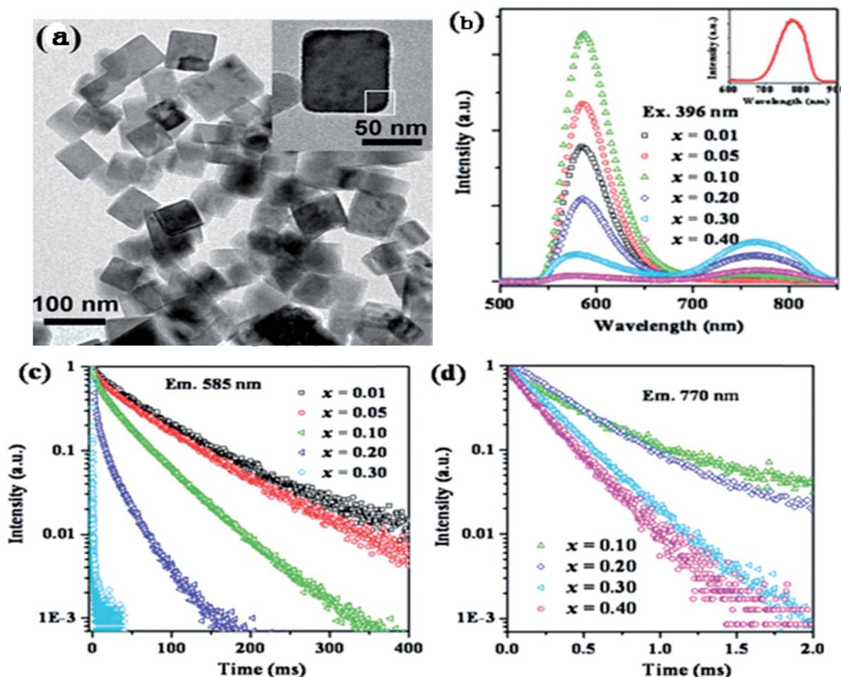
Fig. 10 (a) TEM image of  $\text{KZn}_{0.80}\text{Mn}_{0.20}\text{F}_3$  nanocrystals and a typical nanocrystal (inset). (b) Emission spectra and (c) luminescence decay curves at 585 nm and (d) 770 nm for  $\text{KZn}_{1-x}\text{Mn}_x\text{F}_3$  ( $x = 0.01-0.40$ ). The inset in (b) shows the emission spectrum of  $\text{KMnF}_3$ . The emission spectra and luminescence decay curves were obtained upon excitation with 396 nm light.<sup>66</sup>
