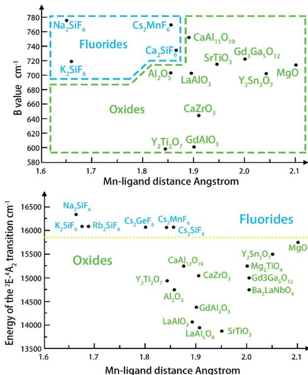
Fig. 4 Relationship between the  $\text{Mn}^{4+}$  ligand<sup>21</sup> bond distance and the Racah parameter  $B$  (top), and the position of the  ${}^2E_g$  level (bottom).<sup>21</sup>
