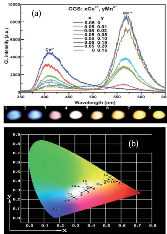
Fig. 15 (a) Emission spectra and luminescence properties of CGS: $x\text{Ce}^{3+},y\text{Mn}^{2+}$  samples. (b) The CIE chromaticity diagram for  $\text{Ca}_2\text{Gd}_8(\text{SiO}_4)_6\text{O}_2:0.05\text{Ce}^{3+},y\text{Mn}^{2+}$  samples under 287 nm UV excitation.<sup>86</sup>
