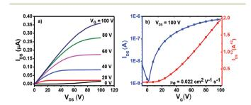
Fig. 4 Output (a) and transfer (b) characteristics of OTFTs based on 4b annealed at 120 °C.
