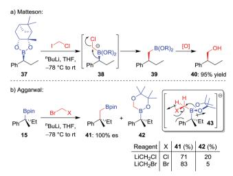
Scheme 8 Stereospecific Matteson homologations of enantioenriched boronic esters. Yield and enantiospecificity of 41 recorded after oxidation; yield of 42 determined by <sup>11</sup>B NMR analysis of the crude material.
