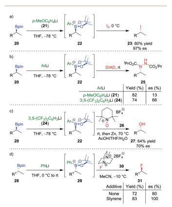
Scheme 5 Stereospecific conversions of secondary boronic esters into other heteroatoms by the reactions of nucleophilic boronate complexes with electrophiles.  $R = CH_2CH_2Ph$ ,  $R^1 = CH_2CH_2C_6H_4OMe$ , DIAD PrO2C-N=N-CO2Pr
