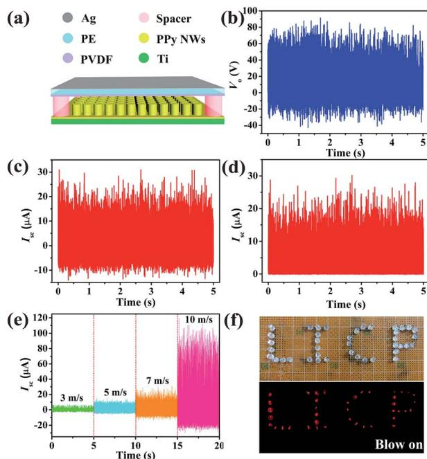
Fig. 5 (a) Device structure of the designed PPy NW-based W-TEG. (b)  $V_o$ , (c)  $I_{sc}$  and (d) the rectified  $I_{sc}$  at a wind speed of  $7 \text{ m s}^{-1}$  (on the scale of 4 BF). (e) The  $I_{sc}$  at different wind speeds from  $3 \text{ m s}^{-1}$  (2 BF) to  $10 \text{ m s}^{-1}$  (5 BF). (f) Photographs of 40 LEDs before and after being powered by the W-TEG.
