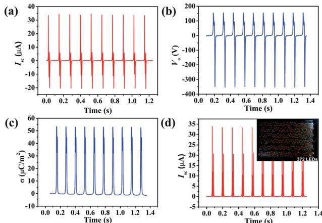
Fig. 3 (a) Short circuit current ( $I_{sc}$ ), (b) output voltage ( $V_o$ ), and (c) charge density ( $\sigma$ ) of the PPy NW-based TENG. (d)  $I_{sc}$  of the PPy NW-based TENG in one direction after rectification. The inset is the photograph of 372 commercial LEDs powered by the PPy NW-based TENG.
