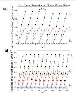
Fig. 4 Time course of water splitting activities of 3 wt% Pt,  $PtO_x$  and 1 wt%  $CoO_x$  Co-modified  $g-C_3N_4$  polymers under (a) UV-vis ( $\lambda > 300$  nm) irradiation and (b) visible light ( $\lambda > 420$  nm) irradiation.
