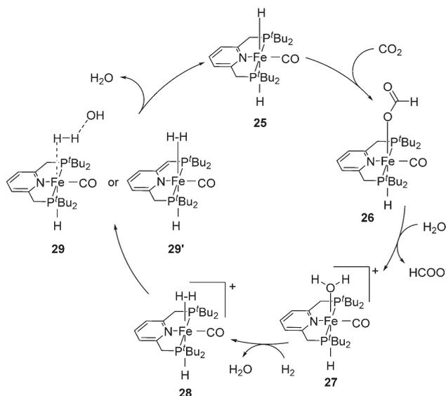
Fig. 12 Proposed mechanism for the hydrogenation of carbon dioxide catalyzed by *trans*-[(<sup>t</sup>BuP<sup>C</sup>N<sup>C</sup>P)Fe(H)<sub>2</sub>(CO)] (**25**).
