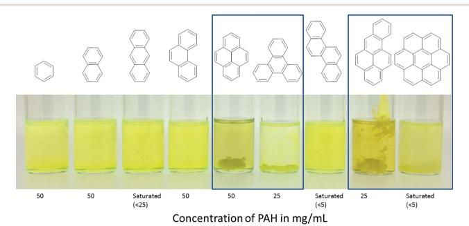
Fig. 3 Effect of the structure of (poly)cyclic aromatic hydrocarbons on the interaction with PIM-1 solution. Three drops of PIM-1 solution (50 mg  $\,$  mL $^{-1}$  in DCM) were added to PAH solutions (in at the stated concentration DCM). The cyclic aromatic hydrocarbons and PAHs tested were (from left to right): benzene, naphthalene, anthracene, phenanthrene, pyrene, triphenylene, chrysene, benzo[a]pyrene and coronene. Blue boxes indicate when precipitation was visually observed.
