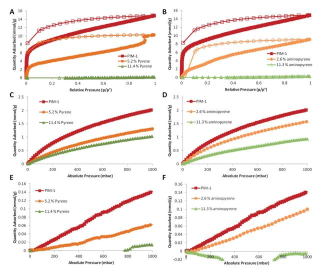
Fig. 9 Gas sorption properties of PIM-1 films post-treated with methanolic pyrene solutions or methanolic aminopyrene solutions. (A)  $\delta$  (B) Nitrogen isotherms (77 K) (legend details the additive content) for pyrene and aminopyrene. (C)  $\delta$  (D) CO<sub>2</sub> isotherms (293 K) (legend details the additive content) for pyrene and aminopyrene. (E)  $\delta$  (F) Nitrogen isotherms (293 K) (legend details the additive content) for pyrene and aminopyrene.
