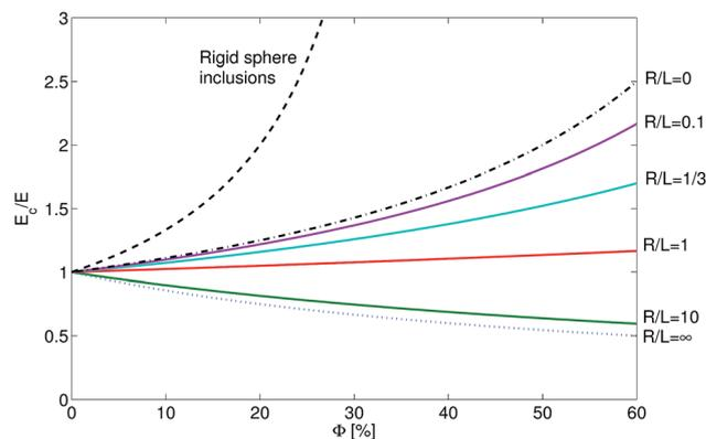
Fig. 4 The stiffness of soft composites. Young's modulus of composites of droplets embedded in linear-elastic solids,  $E_c$  as a function of liquid content. The dotted curve shows Eshelby's prediction without surface tension. The dash-dotted curve shows the surface-tension dominated limit,  $R/L \ll 1$ . The dashed curve shows Eshelby's prediction for rigid spheres embedded in an elastic solid.
