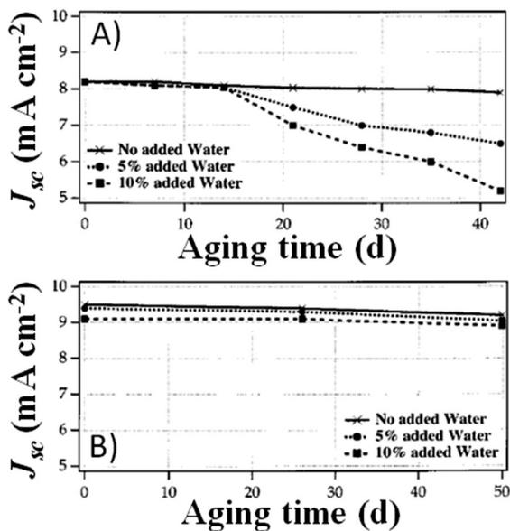
Fig. 17 Long-term stability ( $P_{in} = 0.015 \text{ mW cm}^{-2}$ ) of DSSCs assembled with RTIL-based electrolytes ( $I_2$  10 mM in HMII) encompassing different  $H_2O$  contents. Dyes: (A) N3; (B)  $[Ru(H_2dcbpy)(mhdcbpy)(NCS)_2]$ . Adapted and reprinted from ref. 231.
