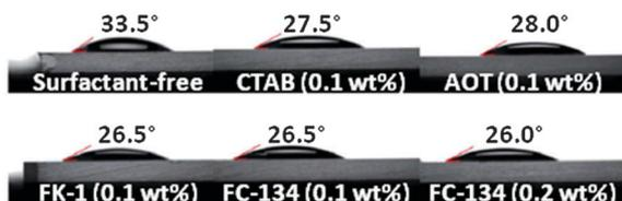
Fig. 11 CA measurements of different aqueous electrolytes at the surface of dye-coated  $\text{TiO}_2$  films. Adapted and reprinted from ref. 163.
