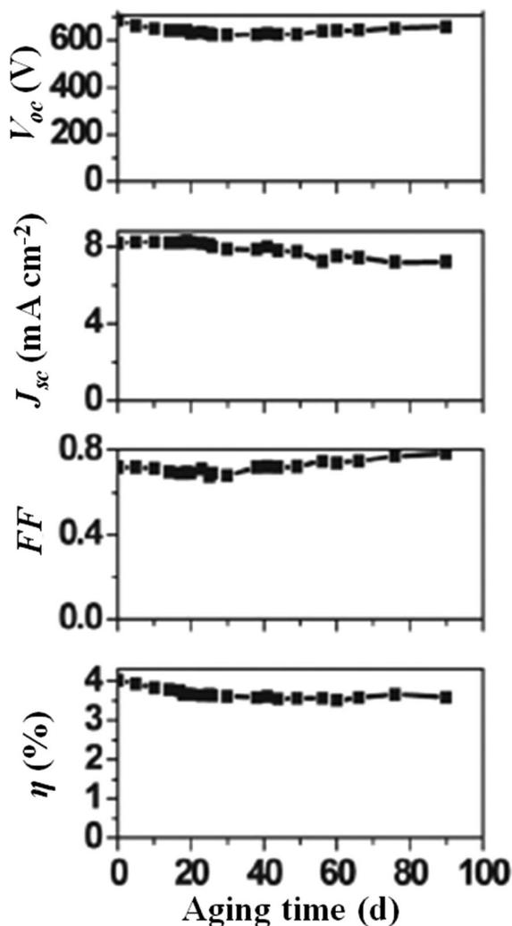
Fig. 14 Long-term stability under dark of a DSSC assembled with an aqueous electrolyte composed of  $[\text{Co}(\text{bpy})_3]^{2+}$  0.20 M,  $[\text{Co}(\text{bpy})_3]^{3+}$  40 mM, NMBI 0.70 M and PEG 300 1 vol%. Dye: MK-2. Adapted and reprinted from ref. 194.
