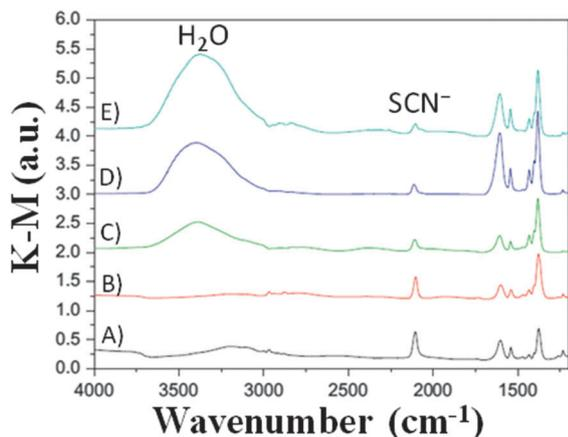
Fig. 5 DRIFT spectra of N719/TiO<sub>2</sub> films immersed in liquid electrolytes (LiI 0.50 M, I<sub>2</sub> 50 mM and TBP 0.50 M in ACN) having different water contents for 192 h: (B) 0 vol% H<sub>2</sub>O; (C) 1 vol% H<sub>2</sub>O; (D) 2 vol% H<sub>2</sub>O; (E) 5 vol% H<sub>2</sub>O. The response of the photoelectrode before immersion is also shown (A) for comparison purposes. Adapted and reprinted from ref. 86.
