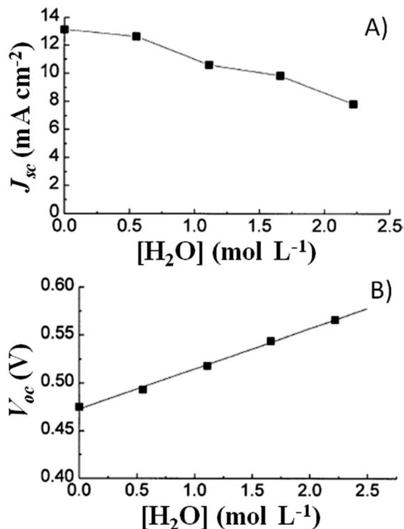
Fig. 3 Variation of  $J_{sc}$  (A) and  $V_{oc}$  (B) values, measured at 0.82 sun, due to water addition in the liquid electrolyte. Electrolytes: LiI 0.10 M and I<sub>2</sub> 10 mM in MAN/H<sub>2</sub>O. Dye: N3. Adapted and reprinted from ref. 43.
