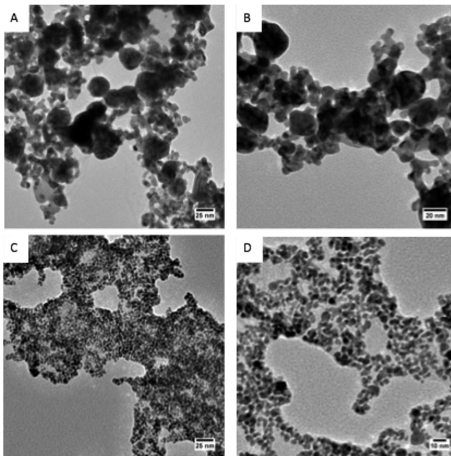
**Fig. 2** Agglomerated vs. aggregated AuNPs. TEM images of 4.0 nm Cit-AuNPs (A, B) and MPA-AuNPs (C, D) immersed in daphnid media for 48 h. Close examination of the aggregated Cit-AuNPs reveal that the AuNPs have formed extended networks of irregular nanowires and large particles. In contrast, the MPA-AuNPs remain dispersed, but closely associated individual AuNPs. Scale bar in (A) and (C) is 25 nm. Scale bar in (B) is 20 nm. Scale bar in (D) is 10 nm.
