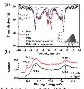
Fig. 2 (a) In-field low-temperature (T = 5 K,  $B_{\text{ext}} = 5 \text{ T}$ ) <sup>57</sup>Fe Mössbauer spectrum of the NZVI@FP nanocomposite. The solid-lines show the three components emerging from the deconvolution analysis. (b) Comparison of the XPS spectra recorded in the Fe2p region for the NZVI@FP nanocomposite freshly prepared (red pattern) and after ageing in air for one month (black pattern).
