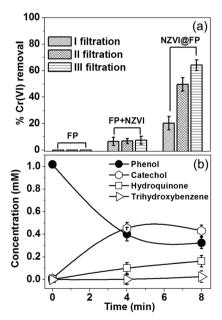
Fig. 3 (a) The Cr(vi) removal performance of bare FP, ex situ synthesized NZVI deposited over FP (3 wt%) and the in situ synthesis of NZVI@FP (5 wt%) as evaluated from 3 filtration cycles. (b) Formation of aromatic compounds as obtained by GC-MS analysis in the phenol hydroxylation process using NZVI@FP (5 wt%) as a catalytic membrane.
