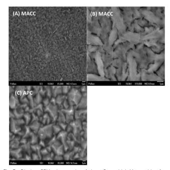
Fig. 3 Displays SEM micrographs of about 5  $\mu$ m thick Mg resulting from galvanostatic plating of Mg onto a Pt working electrode at 1 mA cm<sup>-2</sup>. 0.25 M MACC 2:1 solution in DME is shown at lower and higher magnification in 3A and 3B, respectively. 3C results from 0.25 M APC 2:1 under the same conditions.
