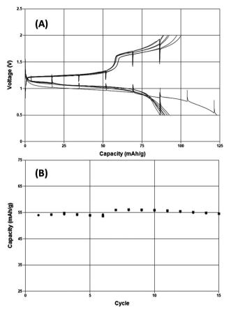
Fig. 4 Galvanostatic cycling of Mo<sub>6</sub>S<sub>8</sub> in 0.25 M MACC 3:2 in DME taken at C/15 for several cycles, shown as a voltage profile in (A) and followed by C/2 for an additional 15 cycles depicted as charge and discharge capacity vs. cycle number (B). Mg serves as the negative electrode.
