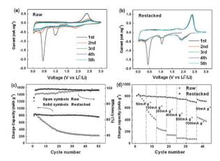
Fig. 3 Electrochemical properties of raw and restacked MoS<sub>2</sub>: cyclic voltammograms of (a) raw and (b) restacked MoS<sub>2</sub> at a scanning rate of 0.2 mV s<sup>-1</sup>; (c) cycling performances at a current density of 50 mA  $g^{-1}$ ; (d) rate capabilities at different current densities (discharge current density was kept at 50 mA g<sup>-1</sup>).
