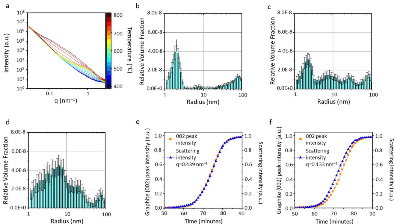
Fig. 5 (a) SAXS data for the heating range 400–800 °C and corresponding particle size histograms for data scans at (b) 700 °C, (c) 750 °C and (d) 800 °C for cellulose- $\text{Fe}(\text{NO}_3)_3$ . Normalised graphite (002) peak intensity alongside scattering intensity at (e)  $q = 0.439 \text{ nm}^{-1}$  and (f)  $q = 0.133 \text{ nm}^{-1}$ .
