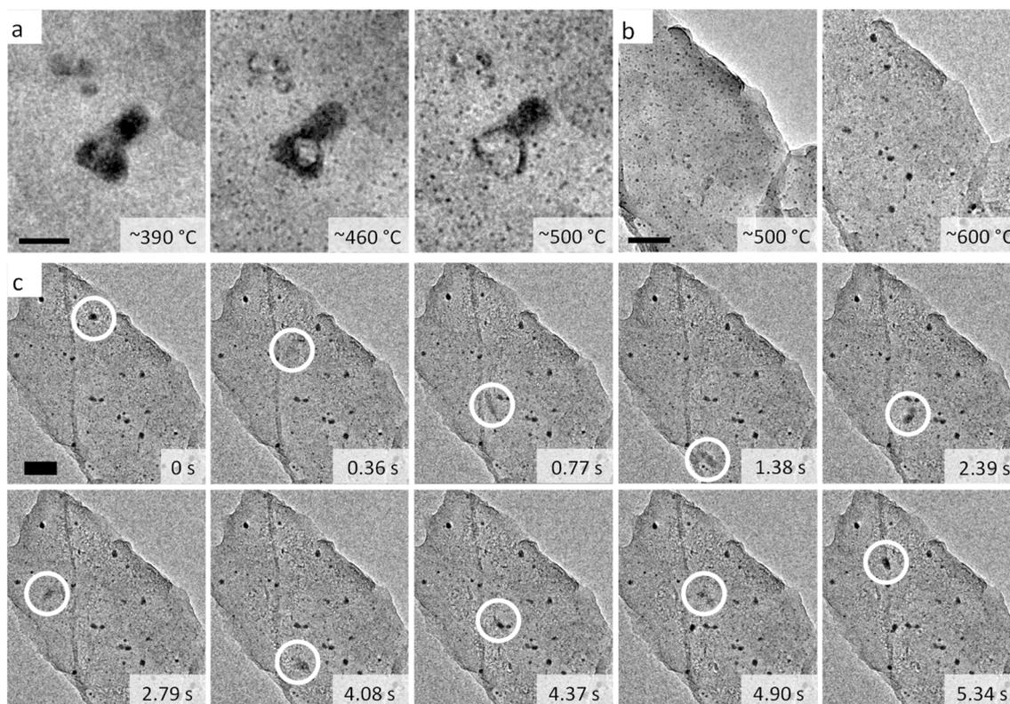
Fig. 3 Snapshots from *in situ* TEM videos showing heating of a cellulose + FeCl<sub>3</sub> sample (a) up to 500 °C (scale bar = 50 nm), (b) from 500 °C to 600 °C (scale bar = 100 nm) and (c) held at 600 °C (scale bar = 100 nm). Circles show the positions of a single particle as it moves.
