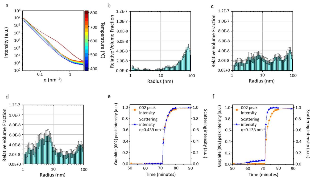
Fig. 6 (a) SAXS data for the heating range 400–800 °C and corresponding particle size histograms for data at (b) 750 °C, (c) 760 °C and (d) 770 °C for cellulose- $\text{FeCl}_3$ . Normalised graphite (002) peak intensity alongside scattering intensity at (e)  $q = 0.439 \text{ nm}^{-1}$  and (f)  $q = 0.133 \text{ nm}^{-1}$ .
