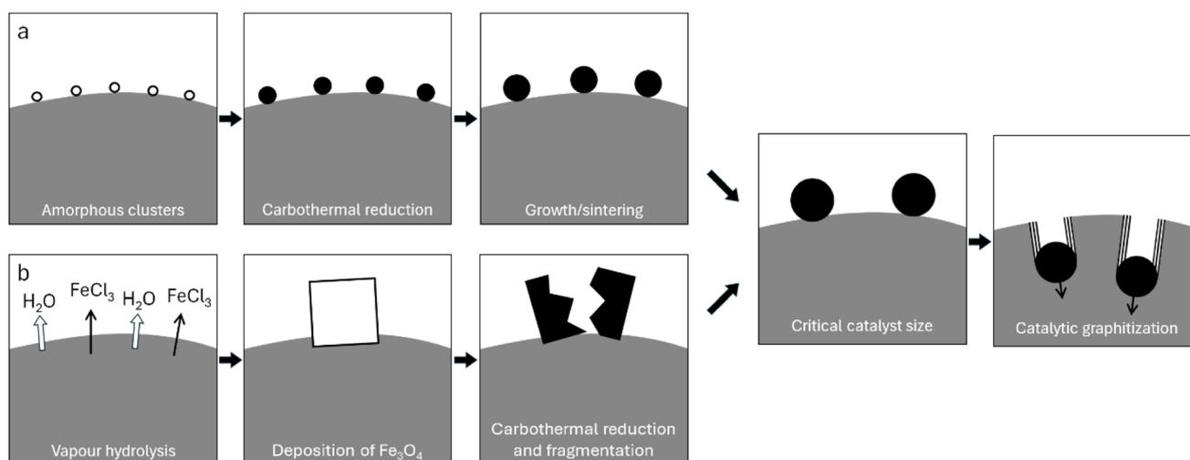
Fig. 7 Schematic showing the two proposed mechanisms of graphitization catalyst formation from cellulose with (a) Fe(NO<sub>3</sub>)<sub>3</sub> and (b) FeCl<sub>3</sub>.
