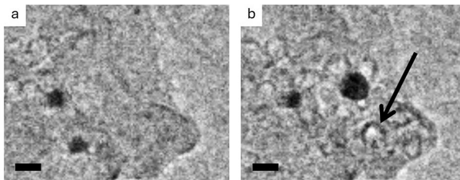
Fig. 4 Snapshots from TEM video showing a region of the cellulose- $\text{FeCl}_3$  sample during the graphitization step, showing (a) amorphous carbon with some Fe nanoparticles and (b) a trail of graphitic carbon nanotubes left by a moving catalyst particle. Scale bar = 20 nm.
