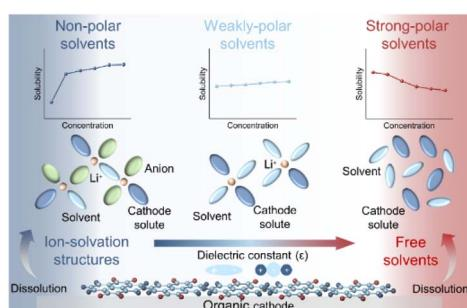
**Revealing the dissolution mechanism of organic carbonyl electrodes in lithium–organic batteries**
