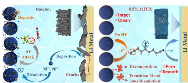
**Multi-functional nitrile-based electrolyte additives enable stable lithium metal batteries with high-voltage nickel-rich cathodes**
