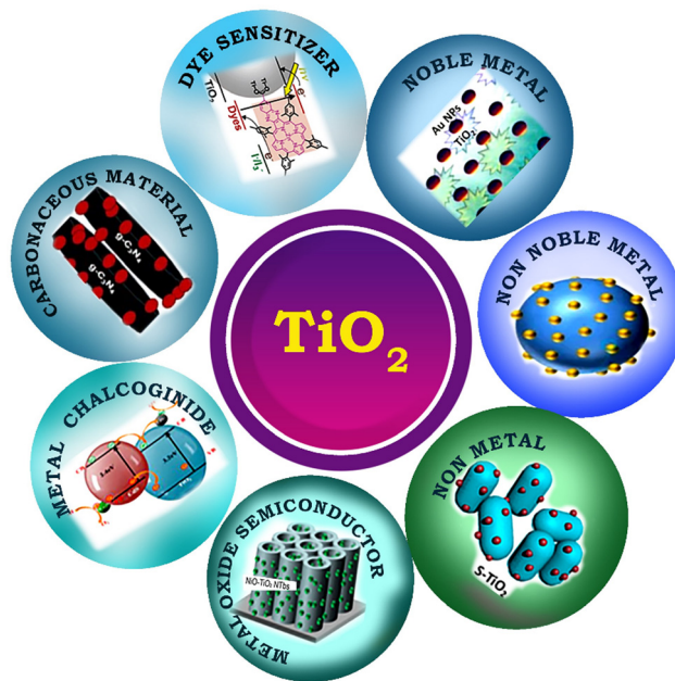
Fig. 3 Schematic representation of different types of chemical components used to improve the photocatalytic efficiency of TiO 2 .
