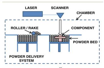
Fig. 4 Schematic of powder bed fusion.<sup>60</sup>
