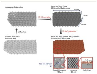
Fig. 10 Schematic of the process for the preparation of a 3D-printed hierarchical porous carbon lattice with MnO<sub>2</sub> deposition.<sup>82</sup>
