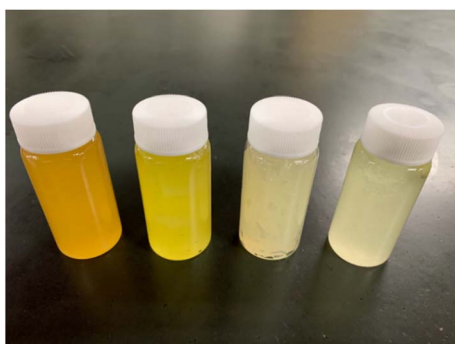
Fig. 16 Nano cellulose dispersion in vegetable oil. From (Left), sesame oil, olive oil, castor oil, soy bean oil. 83
