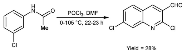
Scheme 43 Synthesis of chloroquinoline analogue.
