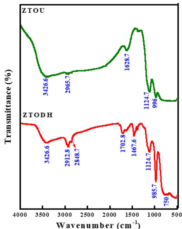
Fig. 8 FTIR spectra of ZTOU and ZTODH nanorods.
