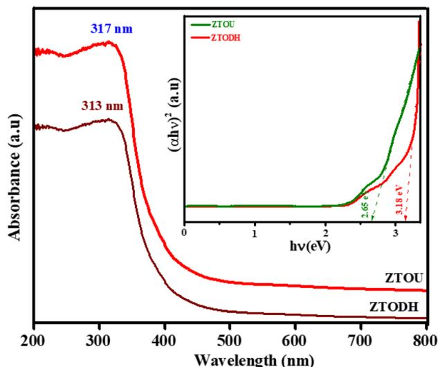
Fig. 10 UV-visible absorption spectra (inset: Wood and Tauc plot) of ZTOU and ZTODH nanorods.
