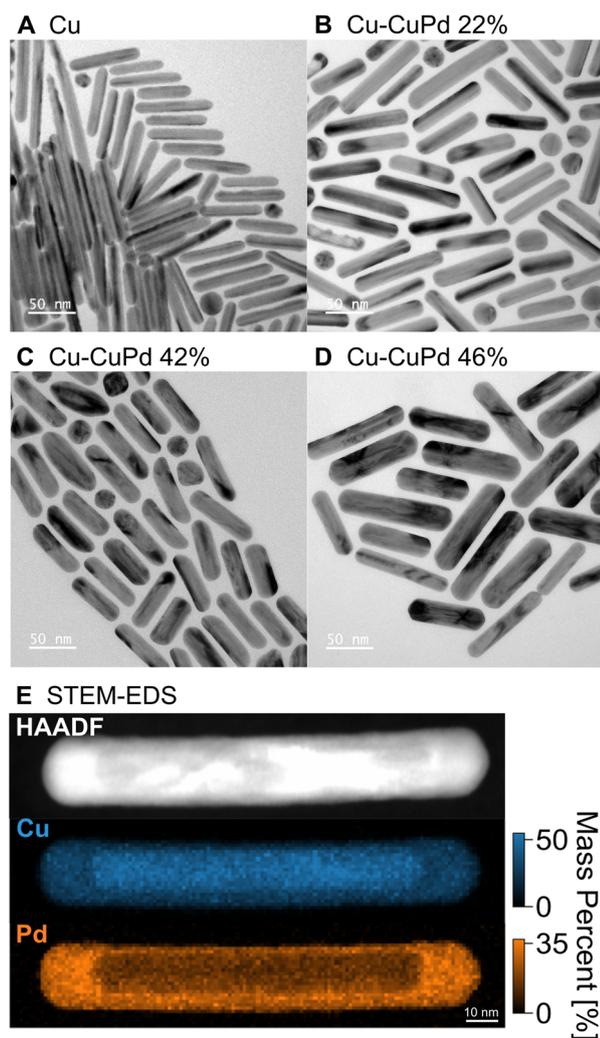
**Fig. 1** Shape and composition of Cu and Cu–CuPd NRs. TEM image of representative (A) Cu NRs and Cu–CuPd NRs with varying concentrations of Pd precursor resulting in NRs with Pd mass percent of (B) 22, (C) 42, and (D) 46%. (E) HAADF signal and STEM-EDS elemental maps for Cu and Pd in a Cu–CuPd NR from the batch containing 46% Pd by mass.
