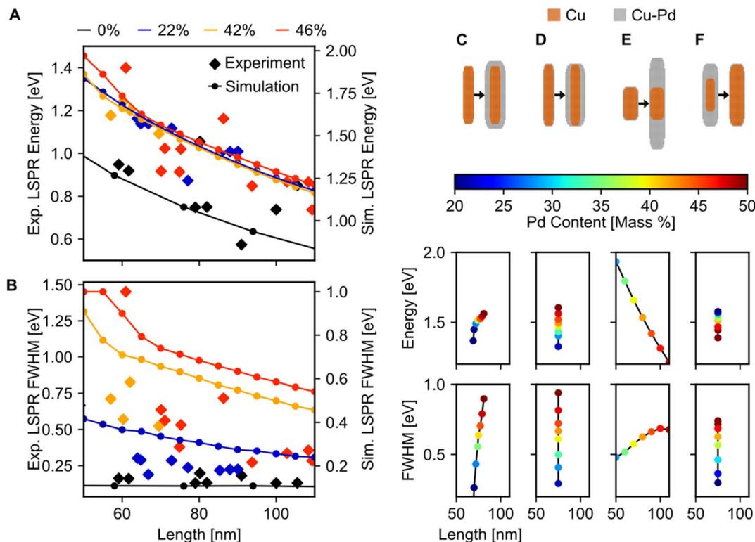
Fig. 6 Effect of Pd content on LSPR energy and FWHM. Dipolar LSPR (A) energy and (B) FWHM for Cu and Cu–CuPd NRs of varying lengths and Pd content, left y-axis experiment, right y-axis simulation. (C–F) Simulations of four different geometries of core–shell growth. Each dot is a separate NR geometry, determined by interpolating between the two indicated schematics above, where marker colour indicates the percentage of Pd in each NR.
