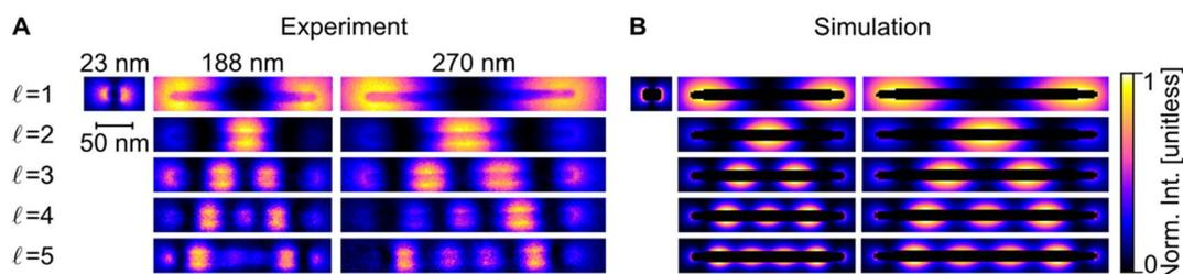
Fig. 3 Longitudinal LSP mode excitation distribution in Cu NRs. (A) STEM-EELS NMF spatial loadings (experiment) and (B) EEL probability maps (simulation) at different energies for the  $\ell = 1 - 5$  LSP modes of three representative Cu NRs of labelled length and width of 12–13 nm.
