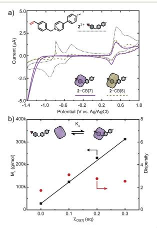
Fig. 5 (a) Cyclic voltammogram of viologen-containing monomer  $2^{2+}$  and its complexation with CB[n] (n=7, 8) at a concentration of 1 mM using a scan rate of 10 mV s $^{-1}$  in 0.1 mM NaCl solution. (b) Molar mass and dispersity of  $2^{2+}$ -containing copolymers vs. equivalents of CB[7]. Cl $^-$  counter-ions are omitted for clarity.
