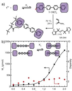
Fig. 3 (a) In situ copolymerisation of DMAAm with  $1^{2^+}$  and CB[7]. (b) Molar mass and dispersity vs. amount of CB[7] in the system. Fitted curve is drawn to guide the eye. Cl $^-$  counter-ions are omitted for clarity.
