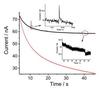
Fig. 6 Chronoamperograms of a carbon micro-disc electrode ( $d=33~\mu m$ ) immersed in a 0.1 M KNO $_3$  (pH = 6.4) solution containing MWCNTs-NH $_2$  (black line) or not (red line) at a potential of 1.90 V vs. SCE. The inset is an enlarged view of impact spike and step at 1.90 V in the presence of MWCNTs-NH $_2$ .
