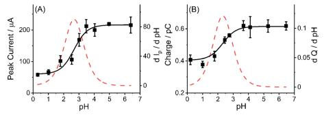
Fig. 8 (A) Relationship between oxidative peak current of MWCNTs-NH<sub>2</sub> modified GCE and pH value of solution; (B) relationship between average charge of oxidative spikes and pH value of solutions in the presence MWCNTs-NH<sub>2</sub> (black square: experimental data; black solid line: simulated curve, and red dotted line: differential curve of experimental data).
