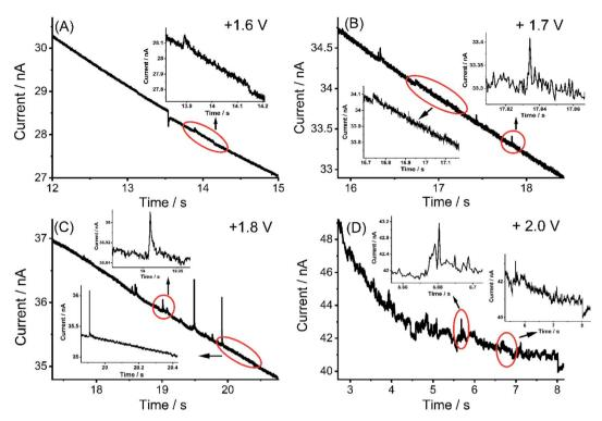
Fig. 3 (A)–(D) Examples of representative chronoamperometric profiles of nano-impact at different potentials (1.60, 1.70, 1.80 and 2.00) in a 0.1 M KNO<sub>3</sub> (pH = 6.4) solution containing 0.01 g L<sup>-1</sup> MWCNTs. No spikes or steps were detected below/at 1.50 V.
