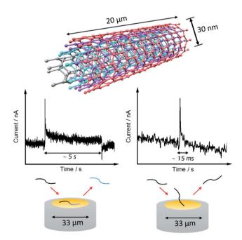
Fig. 4 A schematic view of the possible different collisions of a single MWCNT on the micro-disc electrode ( $d=33~\mu m$ ) associated with the spikes and steps.
