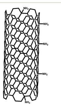
Fig. 9 Schematic structure of the single layer of MWCNTs-NH<sub>2</sub>.
