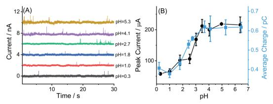
Fig. 7 (A) Representative chronoamperograms of a carbon micro-disc electrode immersed in a 1.0 M (pH = 0.3) and 0.1 M HNO<sub>3</sub> (pH = 1.0) and 0.1 M KNO<sub>3</sub> solutions at different pH values of 1.8, 2.7, 4.1 and 5.3 containing 0.01 g L<sup>-1</sup> MWCNTs-NH<sub>2</sub> at a potential of 1.90 V vs. SCE; (B) the comparison of oxidative peak current from CV (black dots) and average charge from oxidative spikes (blue dots) as a function of solution pH.
