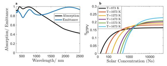
Fig. 6 (a) Absorption and emittance with respect to wavelengths. (b) Overall system efficiency with respect to the solar concentration  $(N_s)$  at different temperatures.
