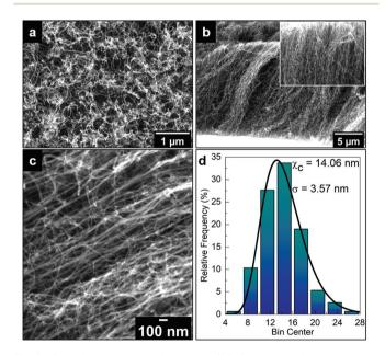
Fig. 1 Scanning electron microscopy (SEM) images of the as-grown vertically aligned carbon nanotubes (VA-CNT). (a) Top-view SEM image showing the tips of the CNT "forest". (b) Side-view SEM image of the VA-CNT showing a height of about to 17 µm. (c) 45° tilt of one of the SEM images used to measure the CNT diameter, whose relative frequency distribution is depicted in (d). (d) From the LogNormal fitting to the distribution, an average diameter of 14.0 nm  $\pm$  3.6 nm was obtained.
