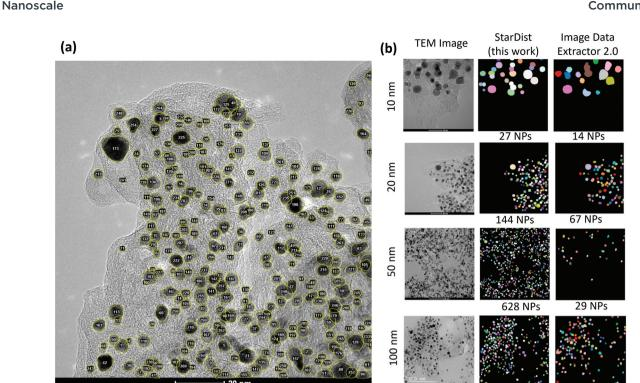
Fig. 5 (a) Localization and counting the particles made available by the instance segmentation approach. (b) Comparison between the predicted segmentation maps of test images at different scales using the StarDist model employed in this work and the ImageDataExtractor 2.0.<sup>64</sup>
